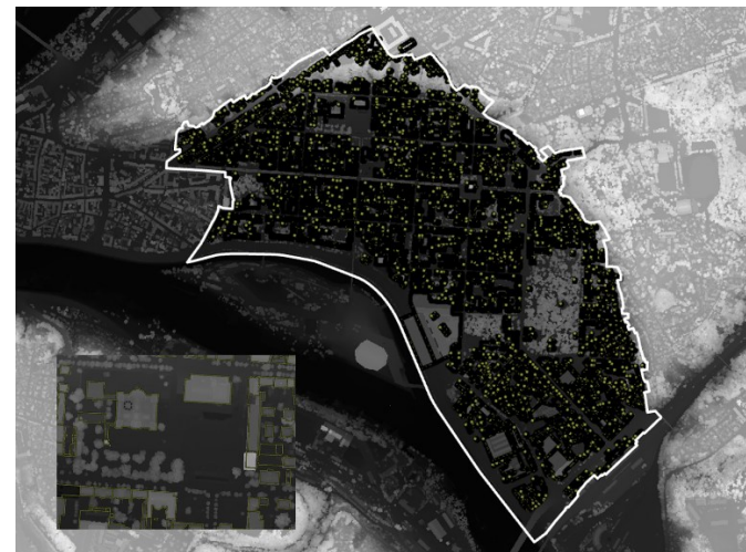
Figure P4. Points generated at a distance of 1 m around each polygon of the building (marked in green).
