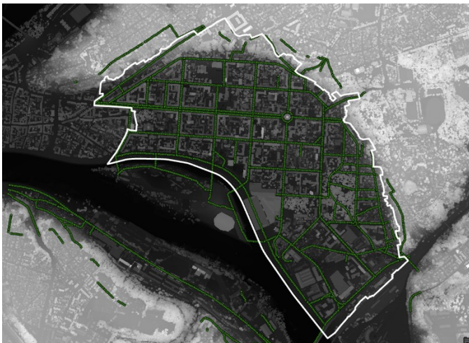
Figure P2. Observation points (marked in green) with a step of 10 meters were generated on all the streets of the study area and some streets outside it, from which this area is visible.
