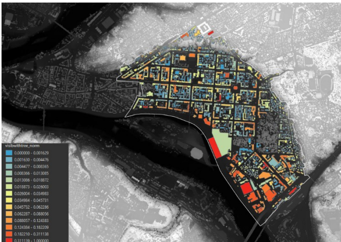
Figure P6. The visibility of buildings as the sum of the visibility points of the façade, normalized by dividing by the maximum value, based on the raster with tree crowns.
